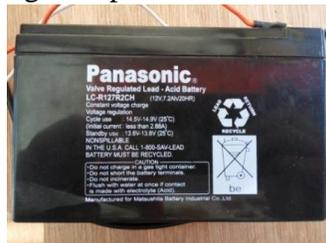
**Gambar 7. Baterai Lead Acid**
