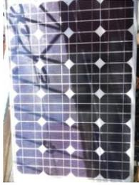
**Gambar 4. Modul Solar Cell**
