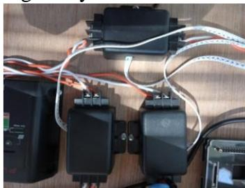
**Gambar 9. Sensor Arus – Tegangan**
